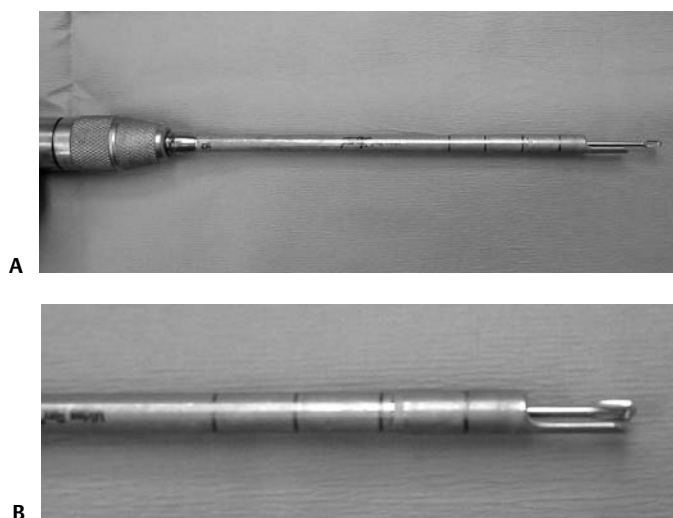
Fig. 1.6 Endoscopic drill with TDQ bit (Midas Rex, Fort Worth, TX) and guard sleeve in (A) extended and (B) retracted positions.
